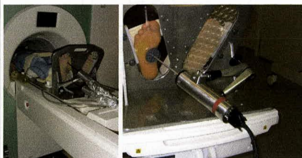
Vibration to the foot sole: amplitude 1 mm, frequency 50 Hz
