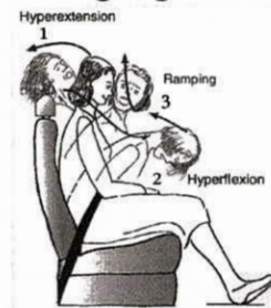
Figure 14.1 Acceleration/deceleration (or whiplash). After a rear-end collision, the occupant is forced backward into the seat back (hyperextension). There may be a vertical motion (called ramping). Following this, the occupant is forced forward as in hyperflexion (see Chapter 15).
