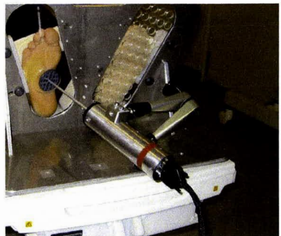
Fig. 1. Vibration probe attached to the subject's arch of the foot with a contact force of 0.05 N to the skin surface. The contact area of the skin surface and the indenter was circular and about 20 cm 2 . The Moving Magnet Actuator System was regulated, so that the contact force was kept constant at 0.05 N throughout the fMRI measurement.
