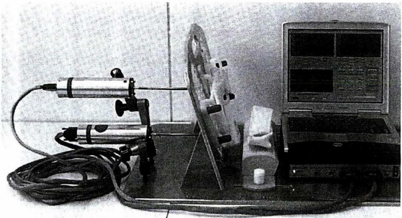
Fig. 1: Moving Magnet Actuator System (MMAS) consists of two intender-vibrators mounted on adjustable stands, a control box and a master and a slave-PC
