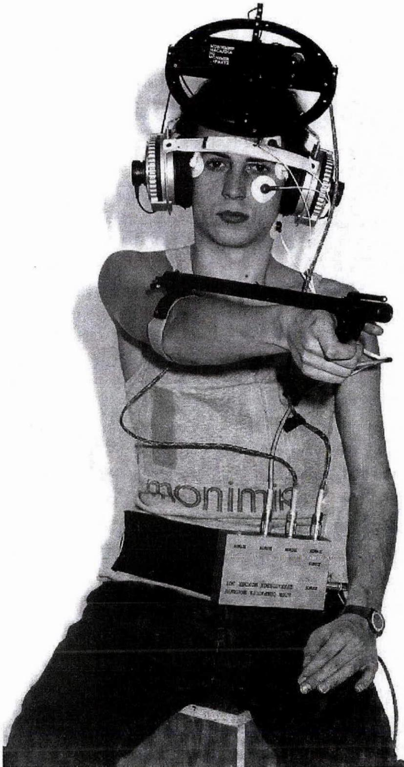
*Fig. 3.* Test person during test with helmet, acoustic system and operator box. For registration of head movements, infrared diodes fixed to helmet, picked up by 2 x 2 infrared scanner cameras. For control of aiming accuracy of head movements and subsequent correction of head positions, a focused light beam (helmlamp) switched on with the gun's trigger. EOG, EMG and EKG amplifiers built into the operator box
