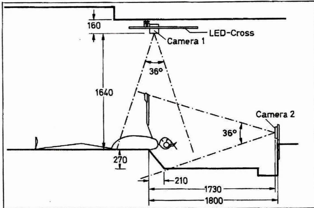
**Fig. 4.** Schematic drawing of test situation in the MIR Space Station. Test person lies on the "floor" of the space station with trunk fixed; head freely moveable above a depression; head (helmet with lamp) and arm movement (arm lamp) registered by 2 x 2 infrared 1D CCD image sensors; cameras mounted in front of face (camera 1) and in body's longitudinal axis (camera 2); visual targets presented on LED matrix mounted with camera system 1
