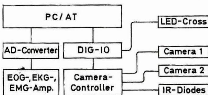
*Fig. 2.* Schematic Diagram of the MONIMIR Equipment
