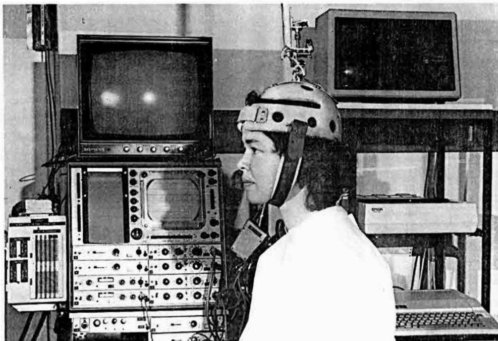
Fig. 3. Apparatus and electronic equipment for the measurement of the movement of head and neck (Reproduced from Berger 1984, by courtesy of the Publisher.)
